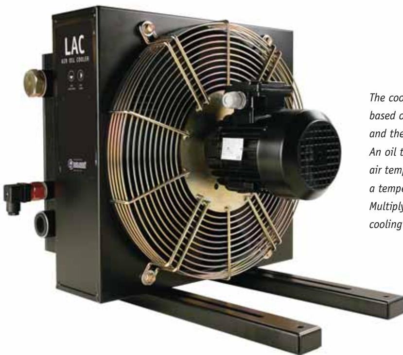
The cooling capacity curves are based on the inlet oil temperature and the ambient air temperature. An oil temperature of 60 °C and an air temperature of 20 °C produce a temperature difference of 40 °C. Multiply by kW/°C for total cooling capacity.
