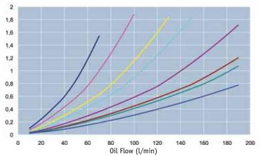
Inlet oil temperature 60°C at  $\Delta p$  max 2 bar Inlet water temperature 20°C
